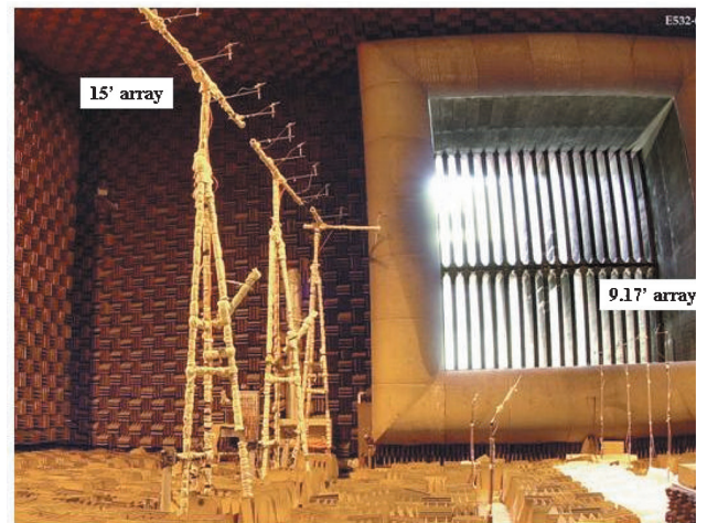
Fig. 16a Photograph of exhaust collector and microphone arrays.
